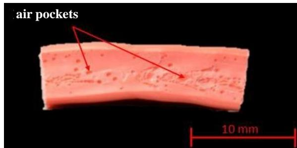
Figure 9: Parts made of ABS showing interlayer defects (Image source: TU-Ilmenau)
