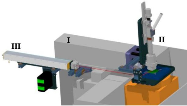
Figure 6: Experimental setup of the hybrid-machine
