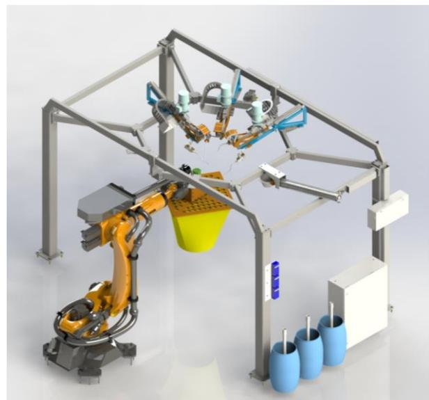
Figure 11: CAD-Layout of the demonstrator setup (Image source: Glamaco)
