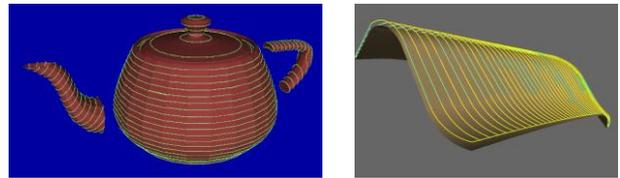
Figure 2: Separation in distinct volumes (left) and freeform surface and z-offset equidistant elements (right)
